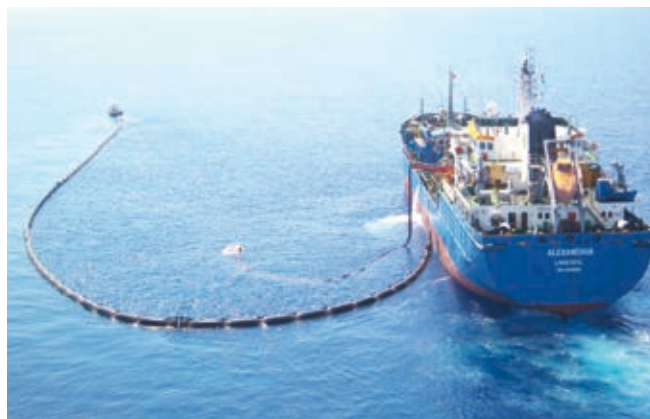
Quarterly drill on board the Alexandria with the deployment of boom and high capacity skimmer
